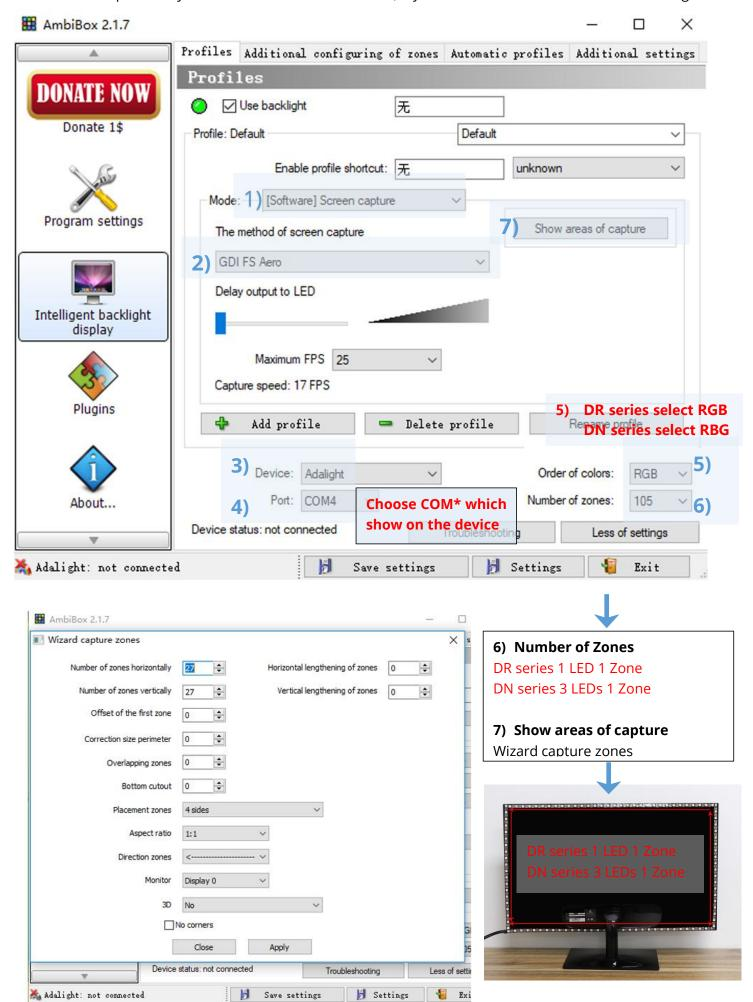
If select correctly you should see Device Status: **Connected**, also down the bottom left it will say Adalight: **connected**.
